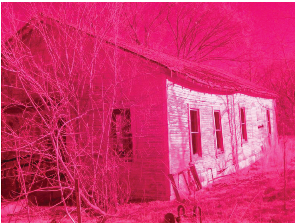
Full-spectrum photography essentially uses the maximum thresholds of a camera's CCD or CMOS sensor to show a visual image not only of the wavelengths of light that we can see with our naked eye, but portions of the UV and near IR spectrums as well.
